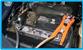
Connect battery cables to vehicle's battery.
