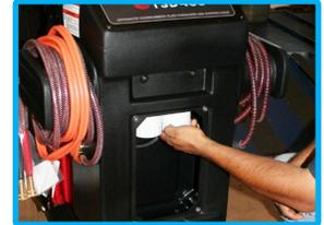
**IMPORTANT:** Machine must be primed after filter change.
