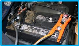
Connect battery cables to vehicle's battery.
