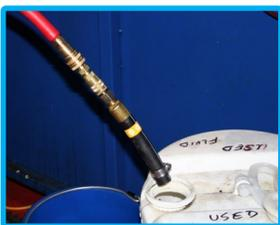
Connect any open end adapter to **red hose** and insert into appropriate disposal container.
