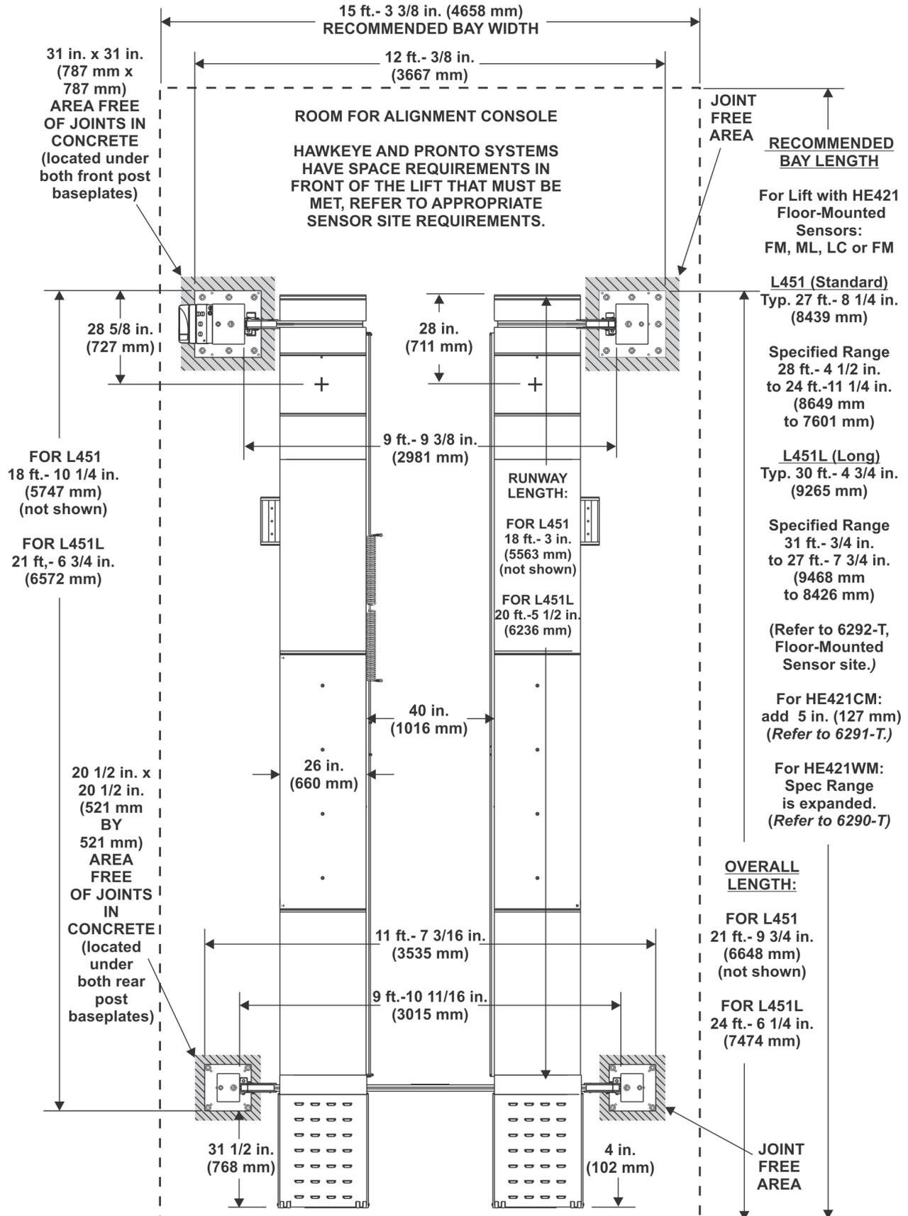
\*If installing over basement or near seams and cracks, refer to Form 4963-T. For exact placement of lag bolts, refer to Form 6530-T.
